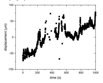
Fig. 5. Time series of the distance fluctuation measured over a total path of 500m in underground corridor. The distance drift is caused by the drift in air temperature. The fast fluctuations are caused by turbulence in air.
