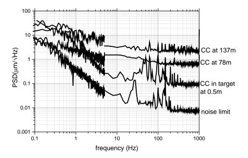
**Fig. 4.** Power spectral density of the longitudinal distance fluctuation for different positions pf the retroreflector. The noise limit is obtained by short-circuiting the circulator and the launching in air. Proc. of SPIE Vol. 10562 105623I-4
