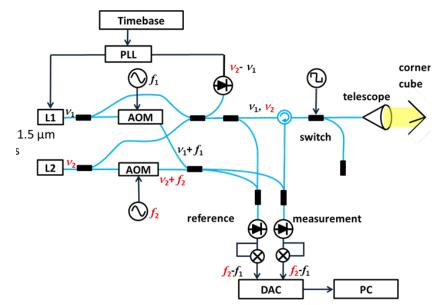
**Fig. 3.** Set-up for the longitudinal metrology. The synthetic wave is generated by mixing two extended cavity lasers in the PM fibers. A superheterodyne detection system is used to measure the phase of the synthetic wave at the fixed frequency of 120 kHz.
