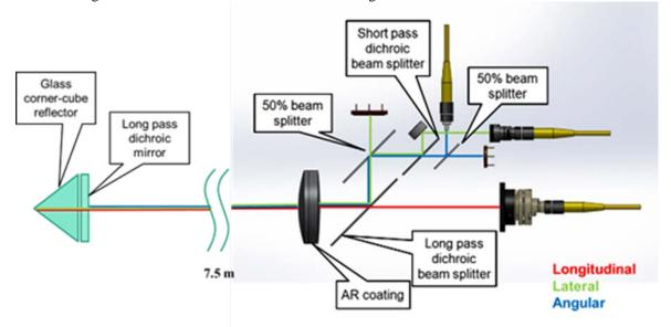
**Fig. 1.** Optical scheme of the attitude sensor. It is formed by the optical head (right) and the passive target (left). The three laser paths are represented in red, green and blue respectively for the 1542, 850 and 780 nm wavelengths
