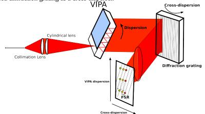
**Fig. 2** : Principle of an échelle-spectrometer based on the VIPA. The optical design is analog to that based on a classical échelle-grating.
