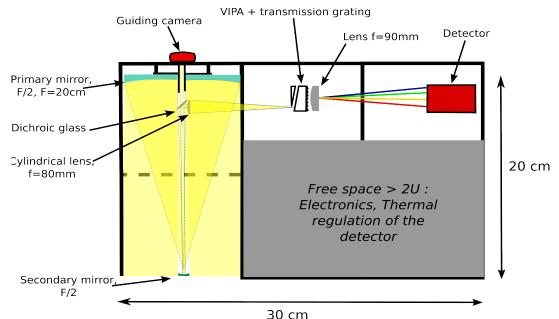
**Fig. 6** : Optical design of NanoVIPA : the spectrometer fits a space inferior to 4U. The remaining 2U can be used to embed the electronics and the thermal regulation of the detector. The Guidance, Control and Navigation (GNC) system could be embedded in a surrounding 6U platform.
