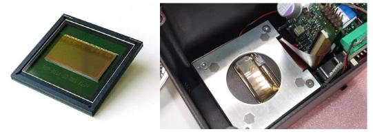
**Fig.** 6. **left**) Pyxalis HDPYX Sensor in BGA, Ceramic Ring configuration; **right**) tested SPOC configuration, a 60nm TiO2 layer has been deposited on plane of plano-convex lens. An optical fiber is set at focal plane of the lens to obtain flat illumination.
