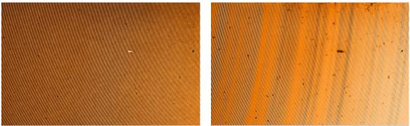
**Fig. 7. left)** Observed Fringes of neon's 703nm spectral line on SPOC; **right**) Observed fringes of whole neon'spectra
