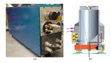
**Fig. 7.** (a) Projected packaging of the 2-μm IPDA laser transmitter. The transmitter is 11.5×26.5×6.4 inch (29×67.3×16.5 cm) in size and weight less than 70lbs (31.75 kg). (b) Schematic of the 2-μm IPDA system. Red lines mark the expended transmitted beam and blue lines mark the return radiation focused onto two detection channels with InGaAs pin and HgCdTe e-APD detectors.
