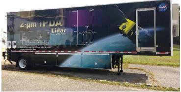
**Fig. 6.** Picture of the mobile lidar laboratory. Located at NASA LaRC, the laboratory is used for IPDA instrument integration and horizontal and vertical pointed ground testing, as well as future field deployment.
