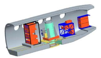
Fig. 8. Projection of the 2-µm triple-pulse IPDA instrument integration inside the NASA B-200 aircraft.
