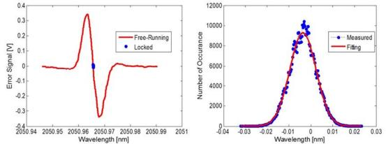
Fig. 5. Comparison of the error signals for the center line locking electronics free-running and locked modes (left). Statistical analysis and Gaussian fitting (right) of the locked wavelength results in wavelength mean and standard deviation of 2050.966967 nm and 0.00913 pm, respectively. This standard deviation translates to  $\pm 650.1$  kHz wavelength jitter.
