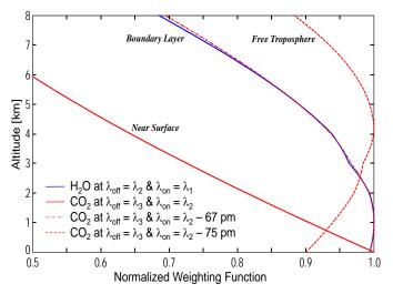
**Fig. 3.** H<sub>2</sub>O and CO<sub>2</sub> pressure-based normalized weighting functions versus altitude at selected spectral positions for an airborne nadir pointing IPDA measurement. H<sub>2</sub>O and CO<sub>2</sub> measurements are weighted to BL and near the surface, respectively, for operating wavelength shown in Fig.2. Tuning CO<sub>2</sub> on-line wavelength 67 and 75 pm away from the selected location optimize the IPDA measurement to within BL or free troposphere.
