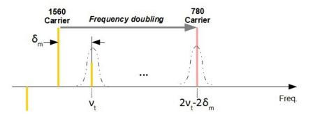
(b) Method used to tune the 780 nm light frequency with respect to the 1560 nm optical link.
