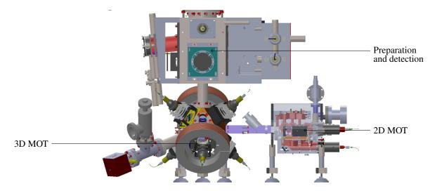
Figure 2: Scheme of the cold atom sources used on the MIGA instrument.
