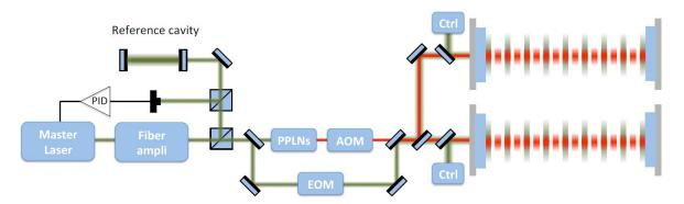
Figure 3: Scheme of the cavities and of the laser system on the MIGA antenna. Adapted from [11].
