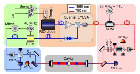
(a) Scheme of the optical bench used on the MIGA preliminary experiment
