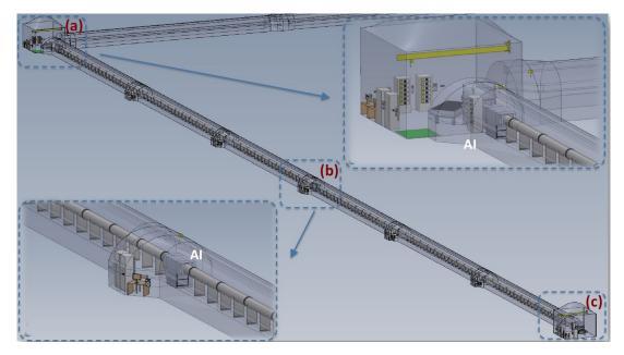
**Figure 4**: Scheme of the infrastructure planned for the MIGA antenna at LSBB. B. The AIs of the initial antenna will be located at (a), (b) and (c). Optical setups for cavity injection will be hosted in room (a). Adapted from [11].
