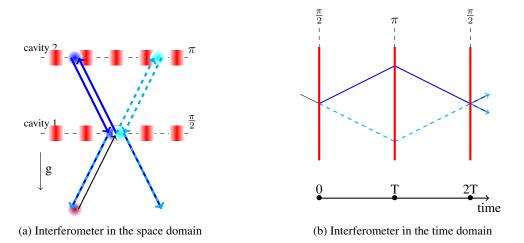
**Figure 1**: Scheme of the interferometers in the space and in the time domain. The dark blue and the dashed light blue lines represent the two arms of the matter-wave interferometer.
