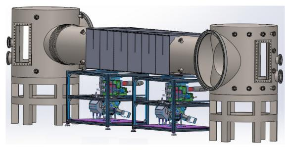
Figure 7: Scheme of the 5 m long baseline gradiometer
