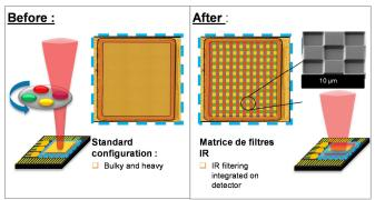
Fig.2: Innovation of pixelated infrared filters on detector
