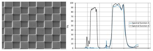
Fig. 3: SEM view of the patterned IR-FPA.
