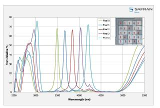
Fig. 4: 5-pixel filter matrix spectral response
