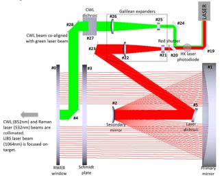
Figure 7: The laser beams (LIBS in red, Raman in green)
