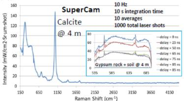
Figure 4: Raman and time-resolved fluorescence spectrum (low resolution example)
