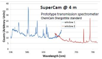
Figure 3: LIBS spectrum (example - only a portion of the spectra is shown)
