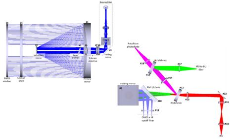
Figure 8: VIS – The collect path (left: telescope and right: beamsplitter) Proc. of SPIE Vol. 10562 105622K-6
