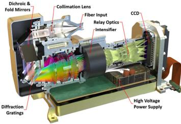
Figure 9: Transmission spectrometer design Proc. of SPIE Vol. 10562 105622K-7
