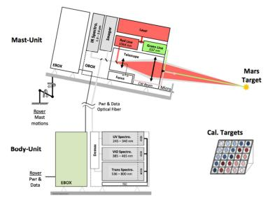
Figure 1: The SuperCam Instrument block diagram
