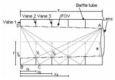
Fig. 3. Ray trace for determining the position of the vanes in the case of diffusely reflecting surface [4]
