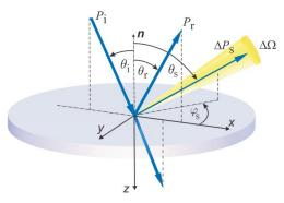
Fig. 1. Geometry for the definition of light scattering and specular quantities: **n** sample normal;  $P_i$  – incident light power at the incidence angle  $\theta_i$ ;  $P_r$  – specular reflected light power;  $\Delta P_s$  – scattered light power into detector solid angle  $\Delta \Omega$ .
