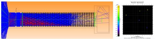
**Fig. 11.** Ray tracing simulation (left) - A lens doublet was placed in the left side of the tube, the detector was placed in the right side. Total irradiance map of the incident flux on the detector (right).
