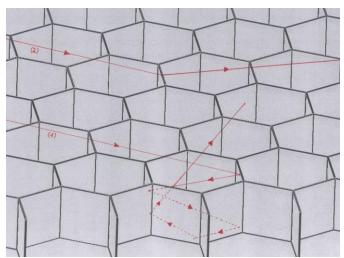
**Fig. 5.** Path of the stray light as reflected from the honeycomb structured surface. Path (1) will lose most of the power after 4 reflection from honeycomb wall (reflection from bottom plane not counted as not coated with Acktar Magic Black<sup>TM</sup>). Path (2) will lose 0.01 of the power and reflected directly to the detector.
