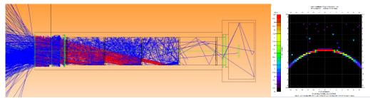
**Fig. 12.** Ray tracing simulation (left) - five vanes were placed in the tube to achieve the same FOV as in the first simulation. The detector was placed in the right side. Total irradiance map of the incident flux on the detector (right).
