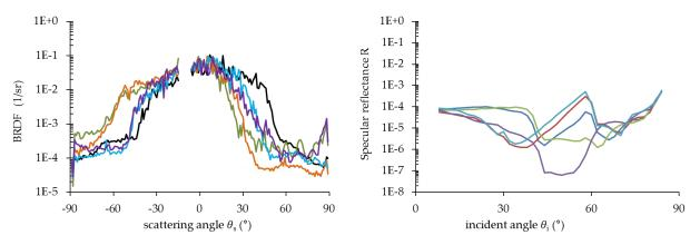
**Fig. 9.** BRDF (left, 10° angle of incidence) and reflectance (right) measurements performed at 5 different measurement positions, respectively
