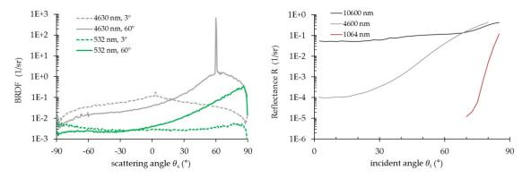
Fig. 2. Left: BRDF measurements at 532 nm and 4630 nm illumination wavelength on a black coating (Acktar Magic Black<sup>TM</sup> [3]) at different incident angles (3° and 60°). TS values were determined to 1% (532 nm, quasi normal incidence) and 15% (4630 nm, quasi normal incidence). Right: Measured specular reflectance (Acktar Magic Black<sup>TM</sup>) as a function of the incident angle for different illumination wavelengths.
