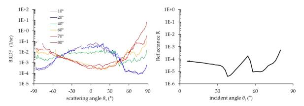
Fig. 10. BRDF (left) and reflectance (right) averaged from 5 different measurement positions, respectively
