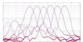
Figure 2: Indicative spectral response of 6 AWG output channels on chip 314-1-436 pre- and post-exposure (X-axis: wavelength, Y-axis: transmission (log-scale). Red and Blue resp., normalized).
