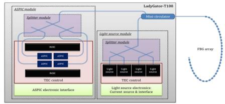
Figure 5: T100 Gator system architecture concept for high performance Thermal Mapping purposes.
