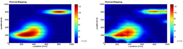
Figure 8: Example Thermal Mapping capability; On the left the original temperature map is displayed, on the right the reconstructed temperature map based on current measurement cabilities. The Temperature range is 120 milli-Kelvin
