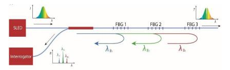
Figure 3: Basic scheme for FBG interrogation of an array of FBG sensors. Each FBG reflects only a specific wavelength.
