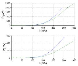
Figure 1: Current vs output power for the two packages pre and post irradiation (blue and green resp.) Top: ESTEC sample 9-40, Bottom: KVI sample 10-16.
