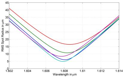
Fig. 3. RMS spot radius within one diffraction order of the AOTF-echelle spectrometer. The wavelength (xaxis) spans across the full width of the detector. Different colors stand for different positions along the slit (the spatial resolution).
