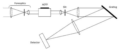
Fig. 1. A simplified optical scheme of échelle-AOTF spectrometer (adopted from [18])
