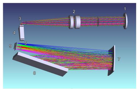
Fig. 2. A simplified optical scheme of the ACS NIR. 1- blocking longpass filter; 2- entry telescope; 3, 6folding mirrors, 4- AOTF crystal, 5- slit, 7-main collimating mirror of the spectrometer, 8- diffraction grating, 9- detector array.
