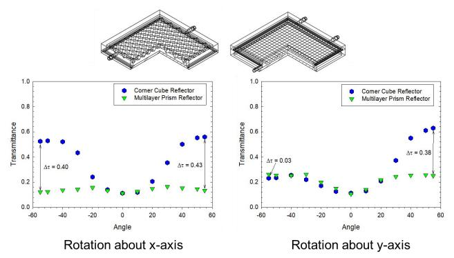
Figure 6: Measurements of the transmission vs. angle of incidence (with air in the cavities) of the published corner-cube design (blue) and crossed-prism design (blue), with angle of incidence along x and y axes.
