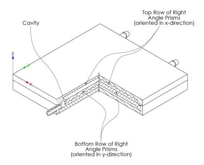
Figure 4: The wide angular response design consists of two 1-dimensional prism arrays with their axes rotated ninety degrees. There are thus 2 cavities.
