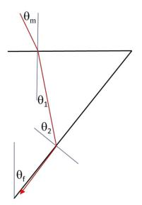
Figure 3: Ray incident on solid corner-cube retroreflector at TIR condition for first facet.
