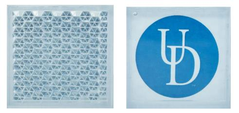
Figure 2: Photographs of corner-cube design with air in the cavity (left), reflective, and (right) with index-matching fluid, becoming transparent revealing logo behind it.
