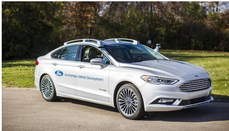
Figure 5: Ford's autonomous vehicle development with integrated LiDAR.<sup>13</sup>
