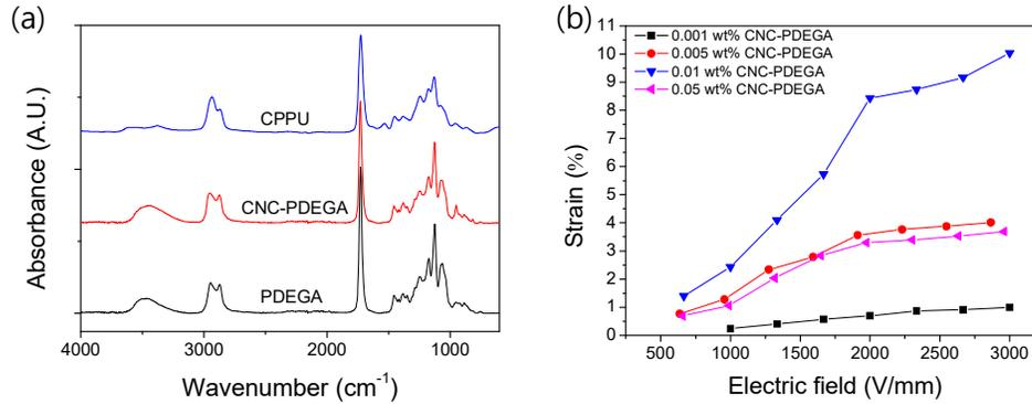
Figure 1. (a) FTIR result spectra of PDEGA, CNC-PDEGA and CPPU and (b) electromechanical strain depending on different electric field and concentration of CNC.
