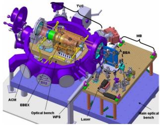
Fig. 10: E-BEX in its testing environment
