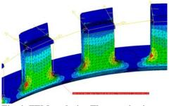
Fig. 4: FEM analysis - Thermo-elastic case
