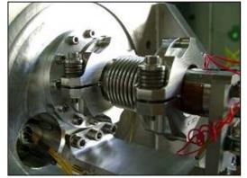
Fig. 7: Metallic bellows with its clamp on the vibration tool
