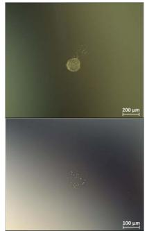
Fig. 2: Typical damage morphologies on E-BEX coating samples: Image (a) correspond to defects appeared after 2 shots at 26.3J/cm<sup>2</sup> on sample 1C28 and Image (b) correspond to defects appeared after 2 shots at 26.3J/cm<sup>2</sup> at 14.3J/cm<sup>2</sup> on sample 1C30.
