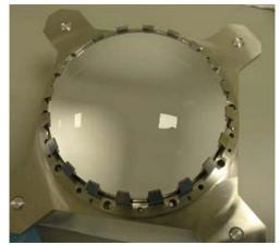
Fig. 3: L3 Lens assembly
