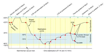
Fig. 4. Schematic overview of thermal vacuum test.
