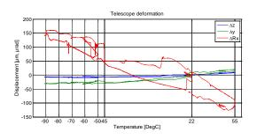
**Fig. 7.** TA-structure deformation as a function of temperature during complete 1<sup>st</sup> thermal vacuum experiment
