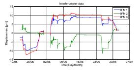
**Fig. 5.** Raw IFM readings during complete 1<sup>st</sup> thermal vacuum experiment
