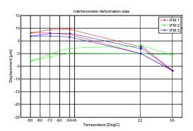
**Fig. 10.** Thermal deformation of the TA-structure results of the re-run of the 2<sup>nd</sup> thermal vacuum test.
