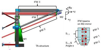
Fig. 3. Schematic overview interferometer monitored paths, TA-coordinate system and measurement positions on M2.
