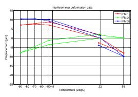
**Fig. 8.** Thermal deformation at stabilization points of the TA-structure results of the 1<sup>st</sup> thermal vacuum test.
