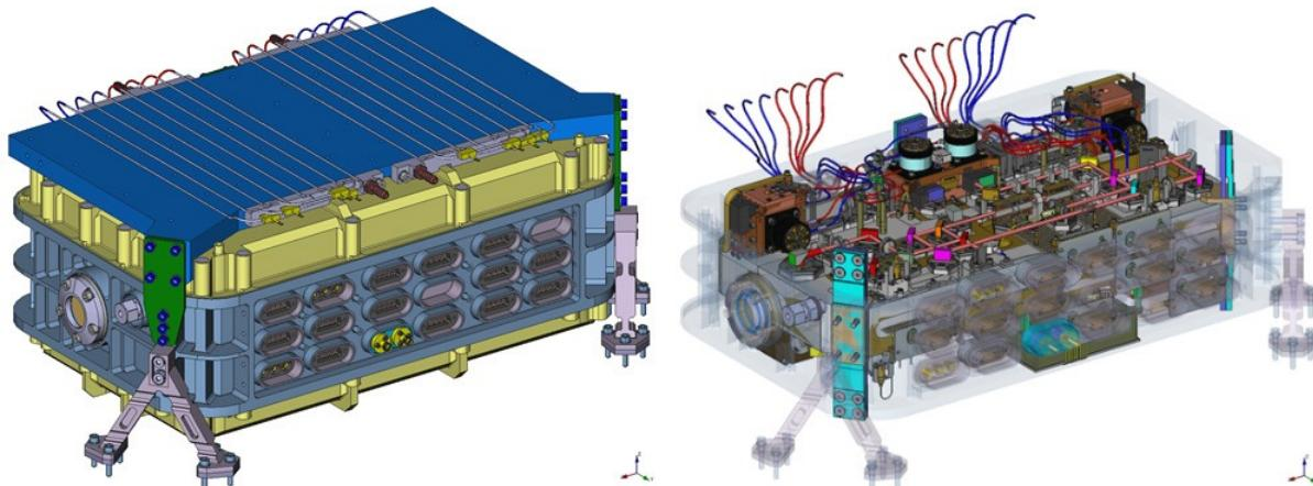
**Fig. 1.** FULAS pressurized housing with top-mounted cold plate and internal optical bench
