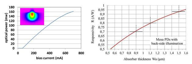
**Fig. 2.** (left) DFB experimental results from various devices within the 1<sup>st</sup> fabrication run and (right) simulation of the back-side illuminated UTC photodiode versus absorber thickness (Wa)
