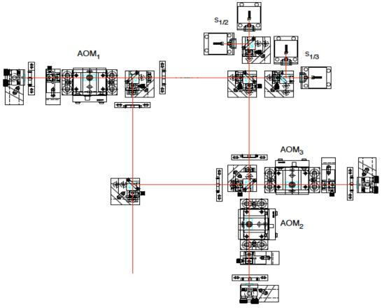
Fig. 2. One module of the optical LOT
