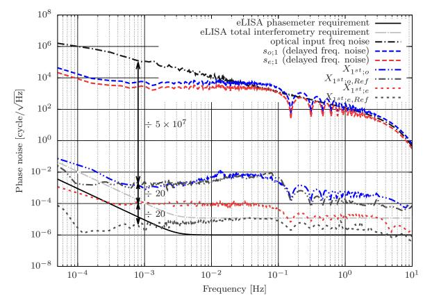
Fig. 6. TDI test with unequal arm configuration
