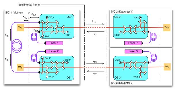
Fig. 4. Principle of the eLISA interferometric measurements
