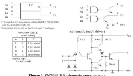
Figure 1. SN75451BP schematic representation.
