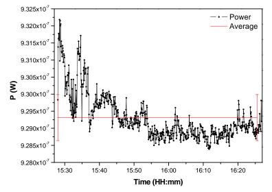
Fig. 9. CAS EP power time evolution measured when a white lamp is supplying the integrating sphere.
