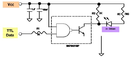
Fig. 2. LED driver: TTL shunt circuit based on an integrated circuit SN75451BP.
