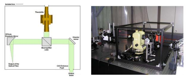
Fig. 3. OGSE-1 schematic representation (left) and real picture (right).
