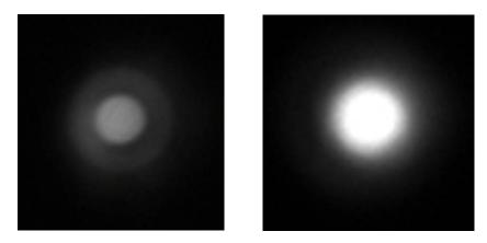
**Fig. 8.** The Spot of UV LED beam at the output of beam-splitter cube. The spot diameter is about 19 pixels (right size image corresponds to a higher exposition time acquisition than the left size one).
