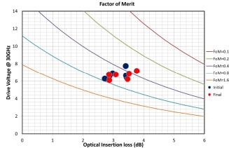
Fig. 7: Figure of merit of the samples before (blue circles) and after (red circles) the tests campaign.
