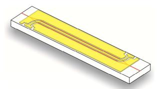
Fig. 3. Microwave electro-optic Mach-Zehnder modulator
