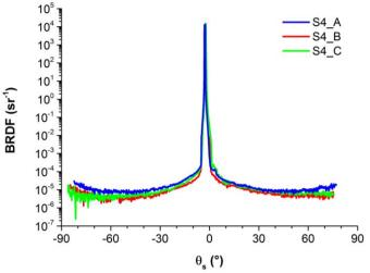
Fig. 7. Scattering of different samples of mirror S4
