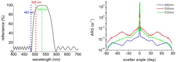
Fig. 9. Rugate filter. Left: Spectral properties. Right: Angle Resolved Scattering at different wavelengths.
