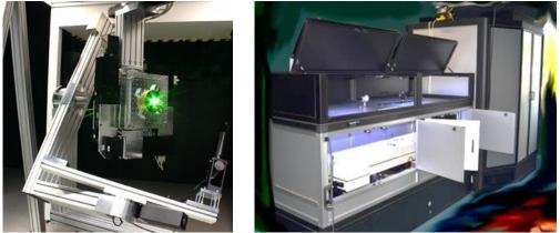
Fig. 1. Light Scatter Measurement Systems ALBATROSS (left) and MARS (right)
