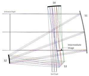
Fig. 6. Afocal Beam Expander (not to scale)
