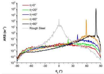
Fig. 4. Scattering of Acktar black coating for different angles of incidence at 4.6 µm
