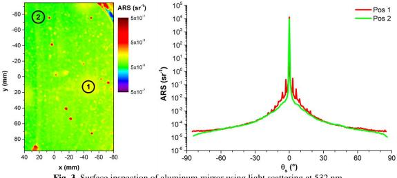
**Fig. 3.** Surface inspection of aluminum mirror using light scattering at 532 nm. Left: Scatter map providing information on roughness, homogeneity, and defects. Right: Angle resolved scatter revealing the origins of enhanced scattering
