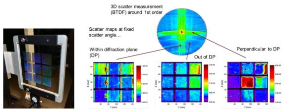
**Fig. 5.** Light scattering analysis of diffraction grating. Left: 3x3 grid of test structures. Right: 3D scattering (BTDF) around 1st order and scatter maps at different locations on scattering hemisphere.
