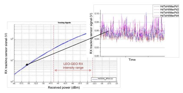
Fig 4: Coherent tracking at GEO-ground RX signal strength (inlay), much below LEO-GEO RX intensity
