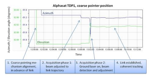
Fig 3: beam steering mechanism position during link acquisition
