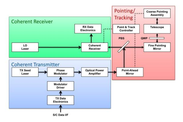
Fig. 1. LCT block diagram.
