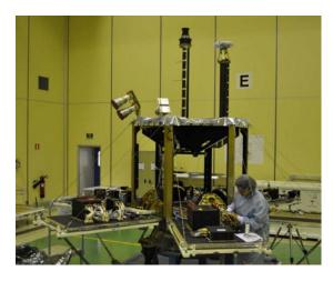
Fig. 2. SEOSAT/Ingenio Flight Platform under integration (Courtesy of Airbus Space & Defence)
