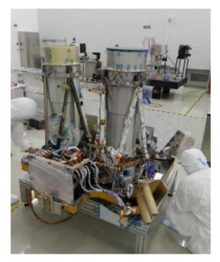
Fig. 7: The SEOSAT/Ingenio Primary payload EQM under integration in ISO-6 (courtesy of INTA)
