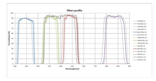
Fig. 6: Transmittance of the SEOSAT/Ingenio filters including spectral shifts at the edge of the FOV
