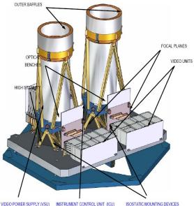
Fig. 3. SEOSAT/Ingenio Primary Payload configuration (Courtesy of SENER) Proc. of SPIE Vol. 10563 105632M-4
