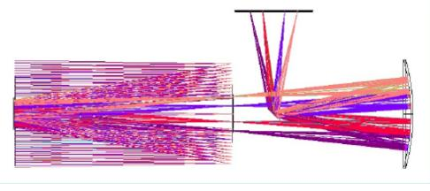
Fig. 4. SEOSAT/Ingenio Korsch telescope optical layout (Courtesy of SENER/INTA)
