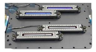
Fig. 5. SEOSAT/Ingenio integrated focal plane (Courtesy of SENER)
