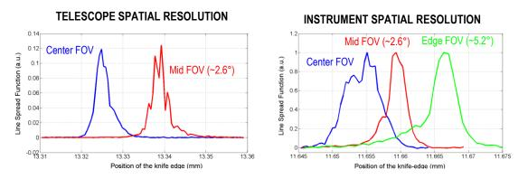
**Fig. 5.** Line Spread Function that is measured at the telescope focal plane in the along-track direction (left) and at the instrument focal plane in the across-track direction (right)
