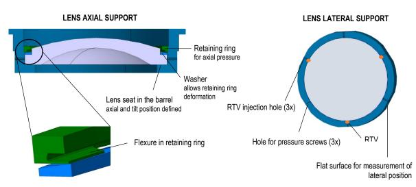
Fig. 1. Lens axial and lateral support
