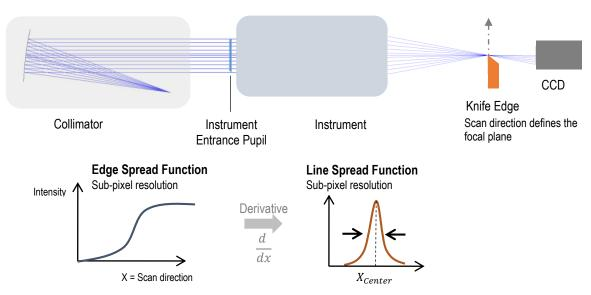
Fig. 4. Principle of the knife-edge test used for instrument spatial resolution measurement
