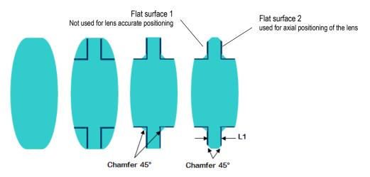
Fig. 2. Flat machining of FIMAS lenses
