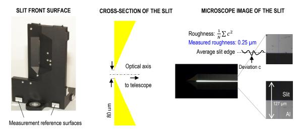
Fig. 3. Pictures of the mechanical slit and microscope view of the edge of the slit
