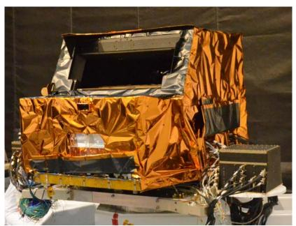
Fig. 8. MSI PFM ready for radiometric tests
