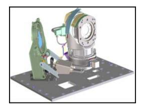
Figure 3 - Gimbal and Latch Assembly
