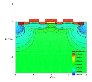
**Fig. 5.** Electron density distribution during reset on a 2D cross-section of the 3D simulated pixel. There is no charge left in the MIGs.
