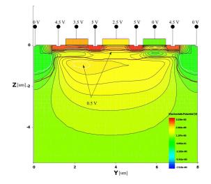
**Fig. 9.** Electrostatic potential distribution in charge transfer potential configuration on a 2D cross-section of the 3D simulated pixel after signal charge electrons have been transferred to the left MIG.
