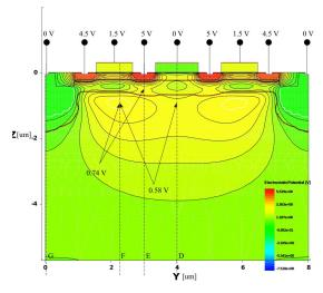
**Fig. 6.** Electrostatic potential distribution during integration on a 2D cross-section of the 3D simulated pixel when 964 electrons are located in the two MIGs (482 electrons in each MIG); the potential barrier from the MIG towards the drain is 0.74 V. The potential barrier between two MIGs is 0.58 V. The potential curves on vertical cut lines D, E, F, and G are depicted on Fig. 7.
