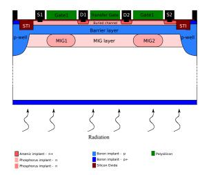
**Fig. 2.** Cross-section of the Double Modified Internal Gate Field Effect Transistor Detector.
