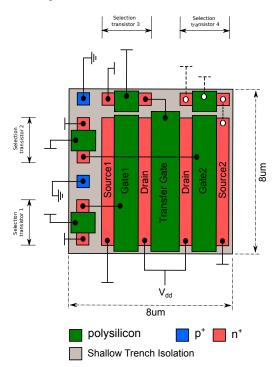
**Fig. 1.** Front side view of the Double Modified Internal Gate Field Effect Transistor Detector.
