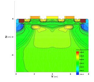
**Fig. 8.** Electron current distribution during integration on a 2D cross-section of the 3D simulated pixel when 964 electrons are located in the two MIGs (482 electrons in each MIG). The interface leakage current is effectively prevented from entering into the MIG layer.
