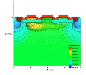
**Fig. 10.** Electron density distribution in charge transfer configuration on a 2D cross-section of the 3D simulated pixel after signal charge electrons have been transferred to the left MIG.
