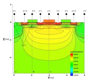
**Fig. 3.** Electrostatic potential distribution during reset on a 2D cross-section of a 3D simulation of the pixel structure. The potential curves on vertical cut lines A, B, and C are depicted on Fig. 4.
