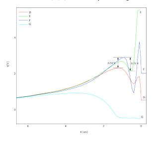
**Fig. 7.** Electrostatic potential during integration on vertical cut-lines D, E, F, and G depicted on Fig. 6. The signal charges in the MIG have a much smaller barrier (0.74 V) towards the drain than towards neighboring pixels (potential maximum of G subtracted from the local potential maximum of F at the depth of around 1 um). This means that vertical anti-blooming mechanism is enabled (excess signal charges flow into the drain and not to neighboring pixels).
