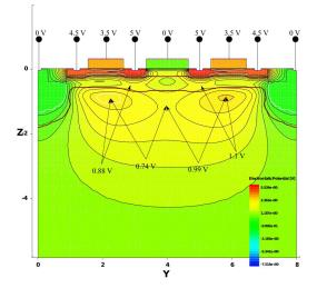
**Fig. 11.** Electrostatic potential distribution in the measurement potential configuration on a 2D cross-section of the 3D simulated pixel. The barrier from the MIG containing 964 electrons to the empty MIG is 0.74 V. The barrier from the MIG containing 964 electrons to the drain is 0.88 V. The barrier from the empty MIG to the full MIG is 0.99 V. The barrier from the empty MIG to wards the drain is 1.1 V.
