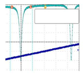
Figure 6: resonance peaks of the hollow core fiber cavity (the dark blue line corresponds to the laser frequency scan). The estimated finesse and contrast are  $F \approx 20$  and  $C \approx 85\%$  respectively.
