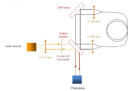
Figure 5: sketch of the resonant cavity and the optical setup used to characterize it. The cavity perimeter is 3.2m, including 3m of hollow core fiber.
