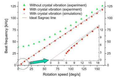
Figure 2. Experimental frequency response curve of our prototype solid-state ring laser gyro with (circle marks) and without (triangle marks) crystal vibration. Also shown (crosses) is the result of numerical simulations in the vibrating crystal case. When the cristal is vibrating, the frequency response curve goes downwards at low rotation rates, similarly to what would be expected for a Helium-Neon ring laser gyro.
