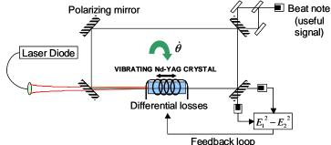
Figure 1. Sketch of our basic experimental setup.
