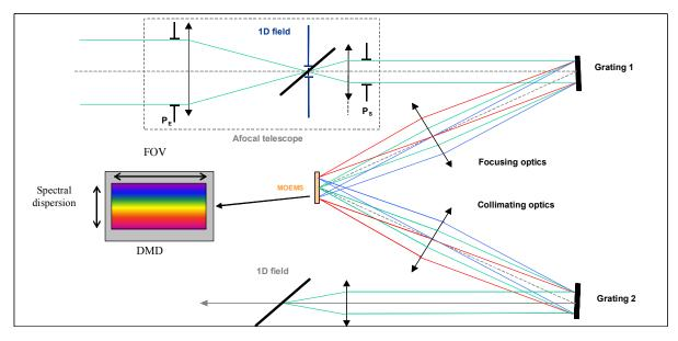
Fig. 1. Principle of the programmable wide-field spectrograph using a MOEMS device (DMD from TI) for wavelength tailoring on each field pixel.
