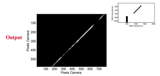
**Fig. 8.** End-to-end measurement: image recorded at the output of the programmable spectrograph; the bright object and the diffraction  $0^{th}$  order light are removed. DMD surface behavior is shown (black pixels are OFF)
