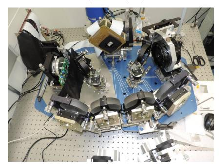
**Fig. 4.** Integrated demonstrator picture Input/OLED is on the left, the DMD at the top, and the output/detector on the right.
