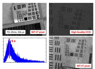
Figure 7. Captured images from the 4T test chip and the measured RMS noise distribution histogram.
