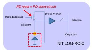
Figure 2. NIT solar-cell mode ROIC pixel structure. It should be noted that the source follower can be replaced by a voltage amplifier too. Proc. of SPIE Vol. 10563 105630J-3
