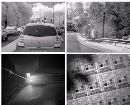
Figure 5. Some example images captured by NIT Solarcell mode InGaAs sensors. Please note the extremely high dynamic range of the arc welding scene.
