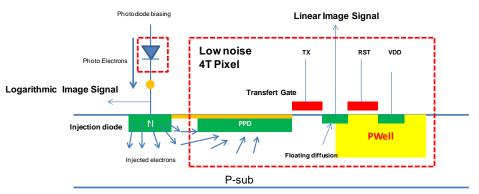
Figure 5. The Injection-Accumulation-Transfer (IAT) ROIC element proposed by NIT.
