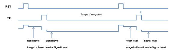
Figure 6. The timing diagram of the ROIC element in Fig. 5. The image signal generated here corresponds to the linear response of the ROIC element.
