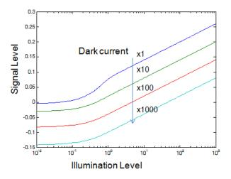
Figure 4. The voltage response of the solar-cell mode photodiode with lateral anti-blooming node (arbitrary units are used here.).
