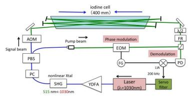
**Fig.2** Schematic diagram of I<sub>2</sub>-stabilized laser YDFA; Yb doped fiber amplifier, SHG; second harmonics generation
