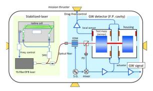
**Fig.1** Conceptual design of DPF Proc. of SPIE Vol. 10563 105632V-2
