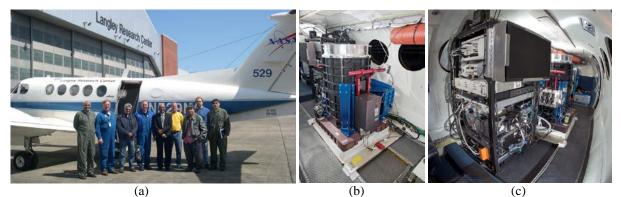
**Fig. 6.** (a) Some team members participated in the 2- $\mu$ m CO<sub>2</sub> IPDA lidar airborne testing in front of the NASA B-200 aircraft. 2- $\mu$ m IPDA lidar instrument (a) and electronic rack (b) integrated inside the aircraft.
