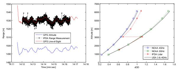
**Fig. 8.** (a) GPS flight altitude corrected to the pitch and roll angles to obtain the IPDA line-of sight compared to the IPDA range measurement. (b) CO<sub>2</sub> differential optical depth versus altitude calculated from NOAA flask sample data and from the IPDA lidar. Results are compared to US standard model calculations.
