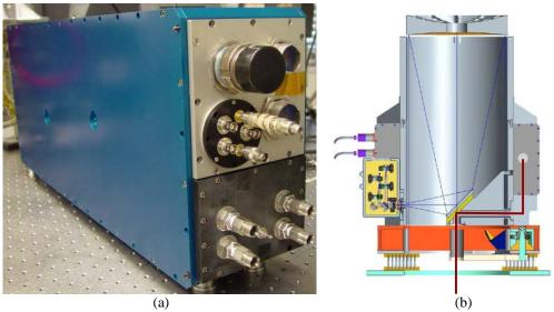
**Fig. 2.** (a) Package 2-µm IPDA laser transmitter. The transmitter is  $11.5 \times 26.5 \times 6.4$  inch ( $29 \times 67.3 \times 16.5$  cm) in size, and weighted less than 70lbs (31.75 kg). (b) Schematic of the 2-µm IPDA receiver system. Red lines mark the expended transmitted beam and blue lines mark the return radiation focused onto the detectors.
