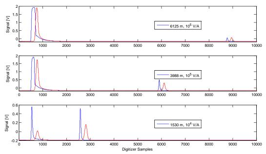
**Fig. 7.** 2-μm CO<sub>2</sub> IPDA averaged on-line and off-line return signals from different altitudes. Data collected using 4 GHz on-line offset and 200 MS/s digitizer sampling rate.
