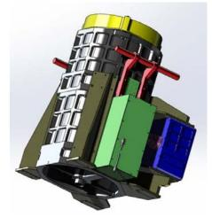
**Fig. 1.** Key components of the 2-μm CO<sub>2</sub> IPDA lidar system. These includes the telescope structure (gray), primary mirror (yellow), laser transmitter box (blue) and beam steering optics (green).
