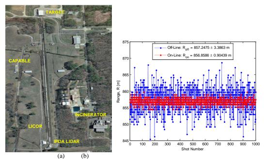
**Fig. 4.** (a) Aerial picture of the 2-μm CO<sub>2</sub> IPDA ground testing site at NASA LaRC. (b) IPDA range determination using both the 2 GHz on-line and off-line wavelengths.
