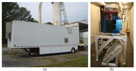
Fig. 3. (a) 35 ft trailer used as a mobile laboratory for hosting the 2-μm CO<sub>2</sub> IPDA lidar for ground testing. A 17 inch widow on the trailer side provides IPDA access to calibrated hard targets. (b) IPDA inside the trailer installed on an aluminium frame. A 45° 24 inch mirror directs the IPDA to the calibrated hard targets.
