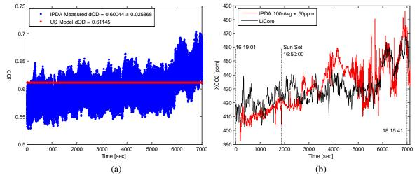
**Fig. 5.** (a) Single-shot  $CO_2$  double-path differential optical depth measurement obtained from the IPDA lidar compared to theoretical value calculated using US standard model. (b) 2 µm IPDA integrated-column  $CO_2$  dry mixing ratio comparison with *in-situ* measurement. IPDA  $CO_2$  dry mixing ratio was obtained using CAPABLE data for differential optical depth conversion after 10 sec averaging. Data collected using 2 GHz on-line offset.
