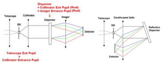
Fig. 2 Classical instrument and constrains on pupil (left) and Double-pass instrument (right)
