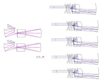
Fig. 11 Concept 2 compliant to OLCI requirements (2 modules) versus OLCI optical design (5 modules) at the same scale
