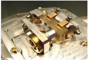
Fig. 8. Cryogenic vacuum CTE measurement setup
