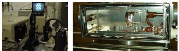
**Fig. 1.** Left: Large aperture WYKO 6000 laser interferometer for wave front testing with a beam diameter of 150mm. Right: Cryostat with 150mm clear aperture window on the left (partly obscured by thermal radiation sheet in this setup). The object being studied is in the center of the cryostat and the cold head with closed cycle is cooler on the right.
