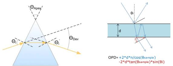
**Fig. 7.** Left: Schematic overview of the minimum deviation refractometry method to determine the index of refraction. Right: Schematic overview of the Fabry-Pérot fringing method to determine the index of refraction.
