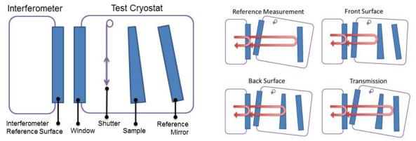
**Fig. 2.** Left: Overview of the setup with the most important components in the interferometer and test cryostat. Right: First a reference measurement is taken without sample. After loading the sample, the reflection of the front surface, the reflection of the back surface, and the transmission of the sample can be measured alternatively in a single cool down run by a slight rotation of the test cryostat.
