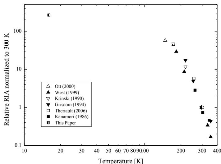
Fig. 4. Ratios of RIA as a function of temperature
