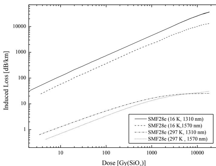
Fig. 4. Radiation-induced attenuation at 300 K and 16 K for two wavelengths in a Ge-doped SMF
