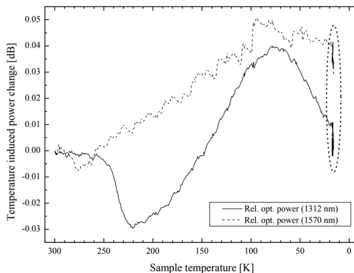
Fig. 3. Temperature induced attenuation in sample fiber in dB between 300 K and 16 K
