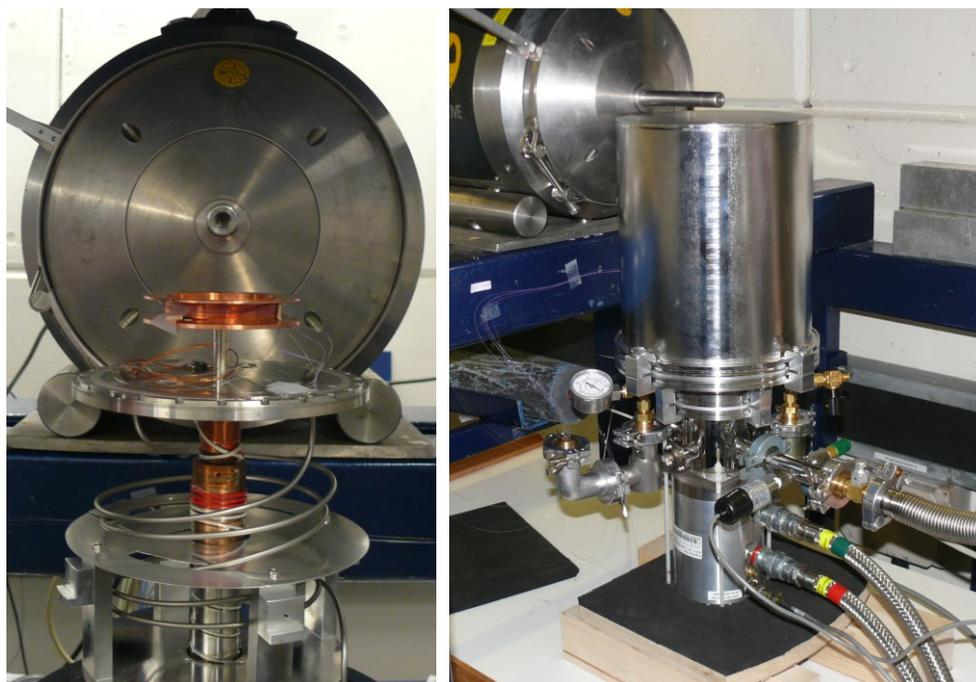
**Fig. 2.** Cryostat open and closed with installed sample fiber at the Co-60 irradiation facility
