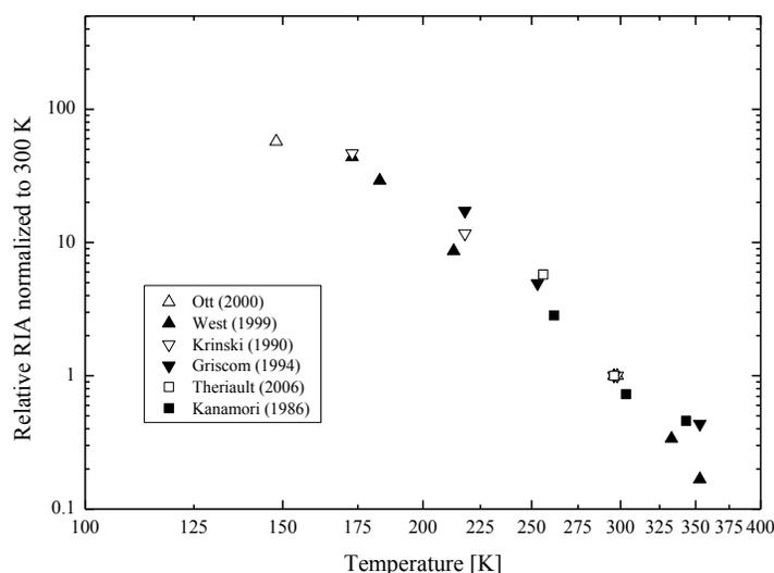
Fig. 1. Overview of temperature dependence measurements of RIA in optical fibers
