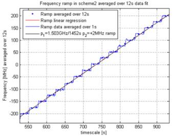
Figure 7 Scheme 2 frequency ramp detail, timescale in (s), Frequency variation wrt to central frequency in MHz, and determination of the best slope.
