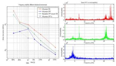
Figure 3 Allan variance and corresponding vibrational spectra for different seismic environments.
