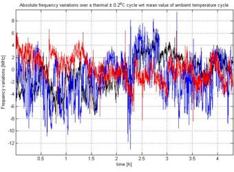
Figure 4 Absolute frequency variations during thermal cycle wrt. ambient T cycle mean value.
