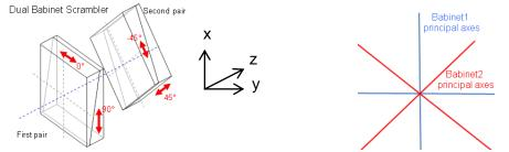
This configuration allows to successively applying 2 phase shifts. To fully understand of these 2 phase shifts, we must notice that each Babinet plate is characterized by 2 systems of axes: First, the system of the birefringent material principal axes, and then the axis of prisms thickness variation. These 2 systems of axes are not necessarily collinear.
