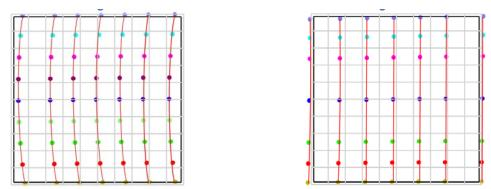
Figure 3 The slit geometry is shown for the two designs presented in Figure 2. By arranging the detector and the slit in the plane of the three mirrors of the TMA, straight slit geometry can be achieved.
