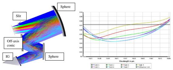
Figure 5 Layout (left) and RMS WFE in waves (right) of the proposed IG based spectrometer after the second optimization step. Diffraction limit is indicated by a horizontal line.
