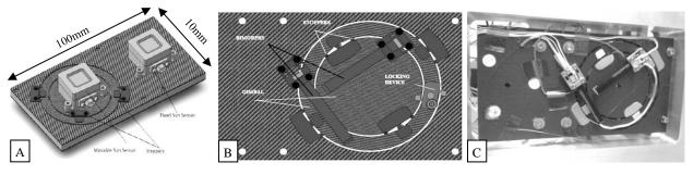
Fig. 2. A) concept design of Optical Bench, frontside, B) concept design of Optical Bench, backside, C) Assembled Optical Bench
