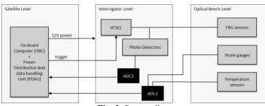
Fig. 3. System diagram
