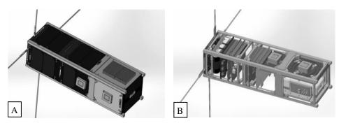
Fig. 1. Nano-Satellite model, A) outside (dimension 30x10x10cm), B) inside
