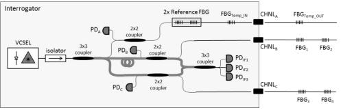
Fig. 4. Schematic drawing of interrogator
