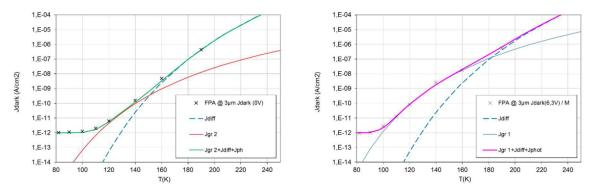
Fig. 8:3  $\mu$ m cut off wavelength APD FPA current measurement in dark conditions at -0.2 V (left) and -6.3 V (right) reverse bias.
