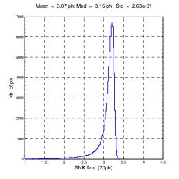
Fig. 6 : example of calculated  $SNR_{Amp}$  histogram of the 3.3 µm cut off FPA from the QEFR and  $N_{deph}$  maps at -8 V and assuming a signal of 20 photons per pixel per frame.
