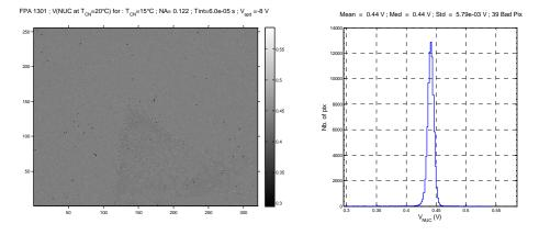
Fig. 3 :  $T_{bb} = 20^{\circ}C$  flat field histogram for 8 Volt of reverse bias (measured Gain of 31) after non uniformity correction with a NUC performed at 15°C.
