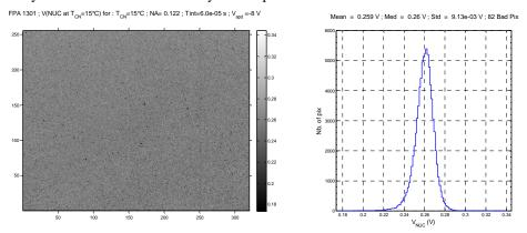
Fig. 2 :  $T_{bb} = 15^{\circ}C$  flat field map and histogram for 8 Volt of APD reverse bias (measured gain of 31) after non uniformity correction. Proc. of SPIE Vol. 10563 1056310-5
