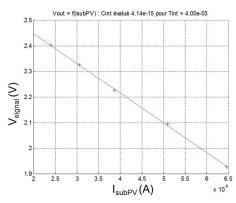
Fig. 1: RAPID FPA integration capacitance evaluation at low APD bias voltage (-0.2 V).
