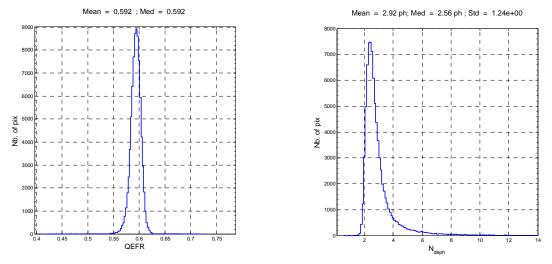
Fig. 4 : QEFR and  $N_{deph}$  histograms of the 3.3  $\mu$ m cut off FPA at -8V ( $G_{meas} = 31$ ).
