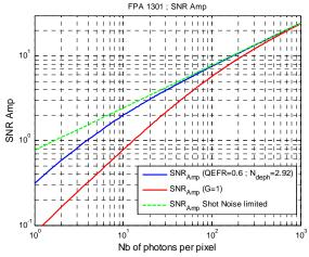
**Fig. 5 :** SNR<sub>Amp</sub> for the 3.3 μm cut off FPA calculated from the mean QEFR and N<sub>deph</sub> measured values at -8V (blue curve). The red curve is evaluated for the same FPA without APD gain (with the measured dark noise unity gain).
