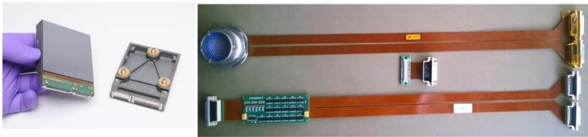
**Fig. 3.** Left: SiC package of 4Kx4K Hawaii-4RG array. Right: 32-channel cryogenic preamplifier and flex cables with hermetic connector for 2Kx2K Hawaii-2RG array.
