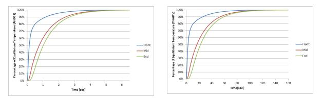
**Fig. 7:** Simulation of the time constant for the transducer made out of aluminum (Al6061, left) and titan (Ti6Al4V, right) respectively.
