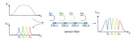
**Fig. 3:** FBG sensor array is illuminated with a broad light source (top left) and the transmission (right side) and reflection spectra (bottom left) are shown.
