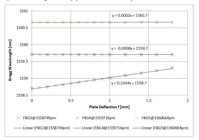
**Fig. 5:** Measurement results of the four-point bending test, FBG3 is the sensor glued directly on the plate, FBG4 is the designed transducer and FBG5 the experimental sensor implemented in the protection hull with vacuum grease.
