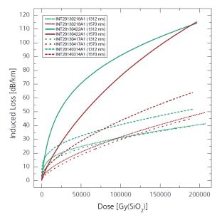
Fig. 9: Radiation test results of the pure silica fibers from four different manufacturers.
