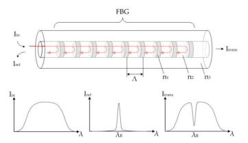
**Fig. 2:** FBG with pitch period  $\Lambda$  and reflected light (top). Bottom, left to right: A broadband optical light is coupled into the FBG, and only light with the Bragg-wavelength is reflected (middle). The transmitted light shows a dip at the wavelength position where the reflection occurs.
