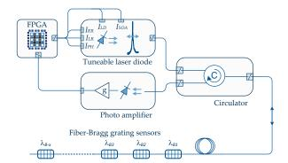
**Fig. 1:** Fiber-optic interrogator based on a tunable laser with control FPGA, optical circulator, fiber-Bragg grating sensors and photo amplifier (photodiode plus transimpedance amplifier).
