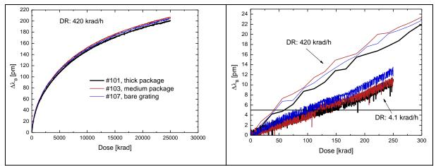
**Fig. 8:** High dose rate (left) and low dose rate (right) TID test of commercial UV-written gratings for different packages.
