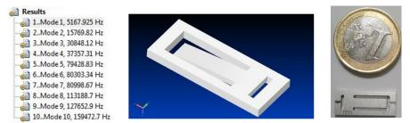
**Fig. 4:** 3D-model of the designed transducer with its Eigen frequencies (left) in the simulation with extreme values. Picture of the final transducer made out of aluminum with respect to the size or a One Euro coin (right).
