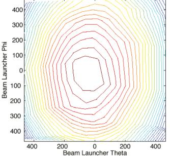
Figure 12: phasemeter output (L) as a function of beamlauncher elevation and azimuth angle. Each contour is 0.002 cycles or 1.3 nm. The central region, near perfect alignment, has a *maximum* in L.  $L\approx 2m$ . Theta, phi: arbitrary units.
