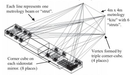
Figure 2: External metrology used to monitor the geometry of SIM to ~100 pm. Geometry means the precise lengths, relative directions and positions of  $D_{1}$ ,  $D_{2}$ ,  $D_{3}$ , the baseline vectors of the three interferometers (science and two reference).
