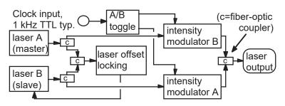
refers only to knowledge of Figure 9: Laser source upgrade for absolute metrology. Light from position changes with respect lasers A and B are held 15 GHz apart by the laser offset locking electronics. A clock signal (in practice, the phasemeter readout clock) toggles intensity modulators A and B. The resulting 500 Hz rate, 15 GHz amplitude FM is fed to the metrology gauge for absolute calibration, as described in the text.
