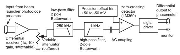
Figure 6: Analog front-end used to convert heterodyne signal to square wave.
