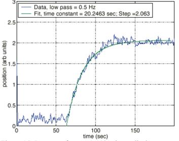
Figure 14: Recovery from a d=110 micron displacement of a corner cube fiducial. L=2 meters. Dither frequency = 50 Hz. Data taken in air.
