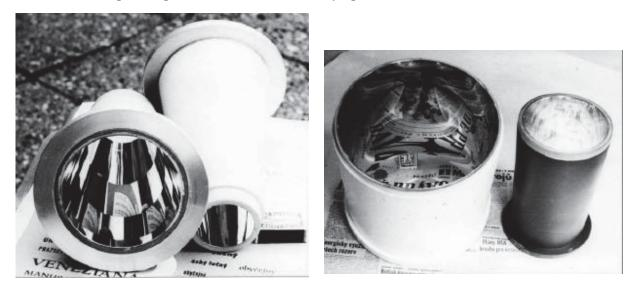
Fig. 2: Mirror shells of the Salyut 7 X-ray mirror assembly, 1981
