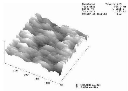
**Fig. 8**: Tapping AFM images of the sample of replicated surface taken in the test facility of the Astronomical Institute in Brera, Italy – the resulting microroughness RMS is 0.3 nm.
