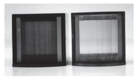
**Fig. 7**: Lobster-Eye telescope prototype, advanced Schmidt arrangement (23 x 23 mm plates with 0.3 mm spacing).
