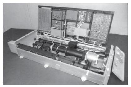
Fig. 5: TEREK X-ray telescope and coronagraph, Fobos 1 spacecraft, 1988
