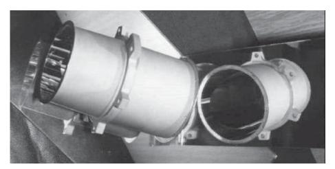
Fig. 1: KORONAS X-ray Wolter mirror, 1979
