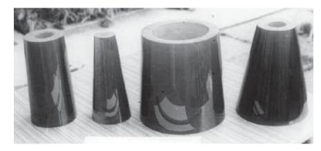
Fig. 3: Mandrels of the double-nested X-ray Wolter 1 mirror, Salyut 7, aperture 240 mm
