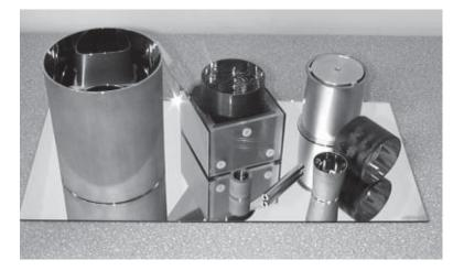
Fig. 6: Replicated grazing incidence X-ray optics
