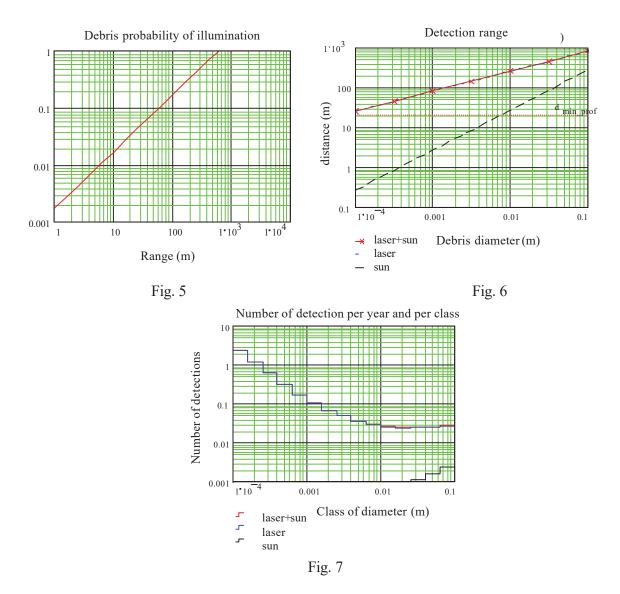
Following this criteria we conclude that the active concept is better suited for small space debris at short range. The return signal is penalized at long range because the return energy is inversely proportional to the range to the fourth power.
