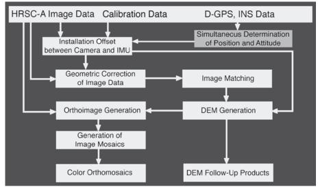
Figure 3. Photogrammetric Processing Line for HRSC-A Data
