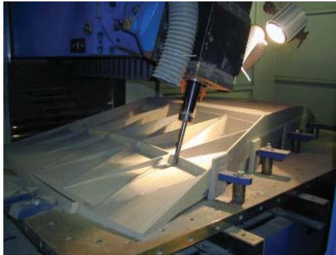
**Figure 3:** BOOSTEC has the capability for CNC milling large parts as shown here with a petal of the FIRST  $\Phi$  3.50 m reflector
