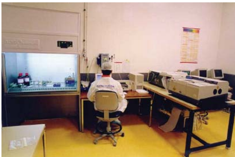
Figure 5 : ASTRIUM Toulouse contamination laboratory with FTIR spectrophotometer
