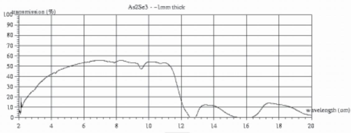
Figure 2 : Spectral transmission of about 1 mm thick  $\text{As}_2\text{Se}_3$  glass. At 10  $\mu\text{m}$ , the refractive index is given to be 2.771 and the Fresnel losses are about 40 % (2.2 dB) for the reflexion on the 2 faces. The intrinsic losses, at 10  $\mu\text{m}$ , are 8% (0.4 dB/mm) for a thickness of 1mm.
