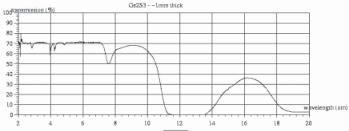
Figure 1 : Spectral transmission of 1 mm thick  $\text{Ge}_2\text{S}_3$  glass. This curve does not represent the intrinsic losses because we need to subtract the Fresnel losses. At 10  $\mu\text{m}$ , the intrinsic losses are estimated to be of 0.5 to 1 dB/mm.
