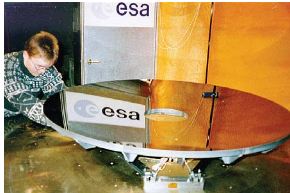
Polishing at Opteon (Finland). The reflector surface was made specular in the visible for allowing a Hartmann test. The surface error was reduced down to 2.5 \mu\text{m} rms (FIRST need).
