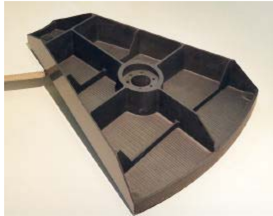
View of a petal as sintered. Note that the rear side lightweighting is performed and completed directly on the green body
