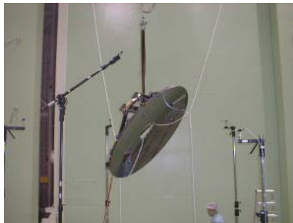
View of the reflector in the LEAF acoustic chamber at ESTEC
